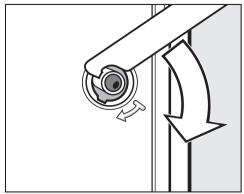
■ Turn the right shipping strut clockwise 90° with the enclosed combination wrench.
